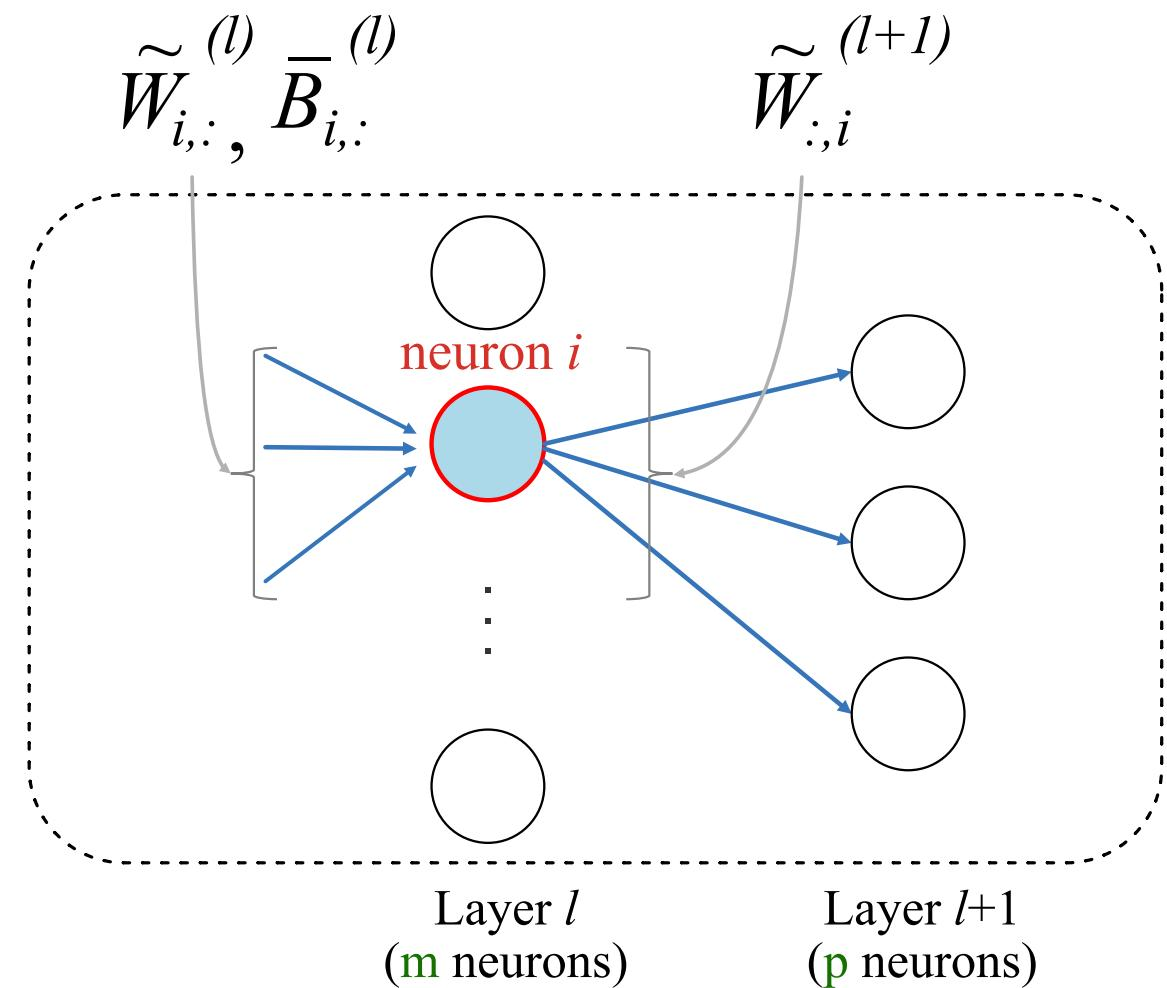
$$\tilde{F}_{i,:} = [\underbrace{\tilde{W}_{i,:}^{(l)}, \bar{B}_i^{(l)}}_{\text{Incoming features}}, \underbrace{\tilde{W}_{:,i}^{(l+1)}}_{\text{Outgoing features}}]$$
